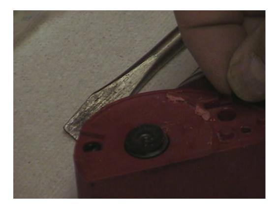
11. Use Dremel or such to cut out inside of blade guard to fit over new blade..
