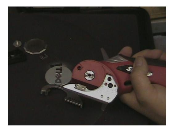
10. The blade guard needs two small o-rings stuck in holes to hold guard out some from the new thicker pinking blade.
